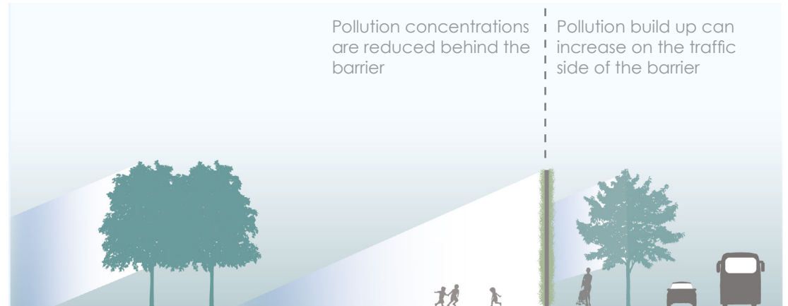
Diagram demonstrating the effect of green screens on pollution adjacent to a road based on Using Green Infrastructure To Protect People From Air Pollution , GLA (2019) © ARUP
