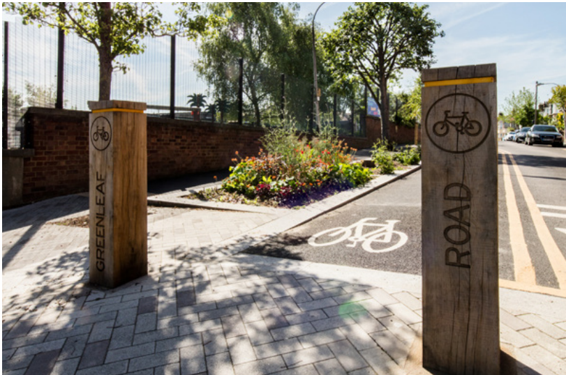
Fixed bollards and planting limits vehicles to one way and retains two way cycle access at Greenleaf Road, Wathamstow. Image photo credit: © Alexander Christie. Scheme design: LBWF Highways in collaboration with what if: projects Ltd.
